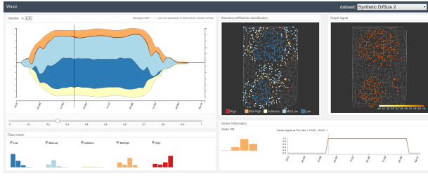
Figure 6: Screenshot of our prototype interface which comprises a stacked graph visualization (top left), threshold slide bar for wavelets coefficients (middle left), average feature vector in each class (bottom left), graph map depicting node labels and function intensity in specific time slice (top right), and time series of a node (bottom right).
