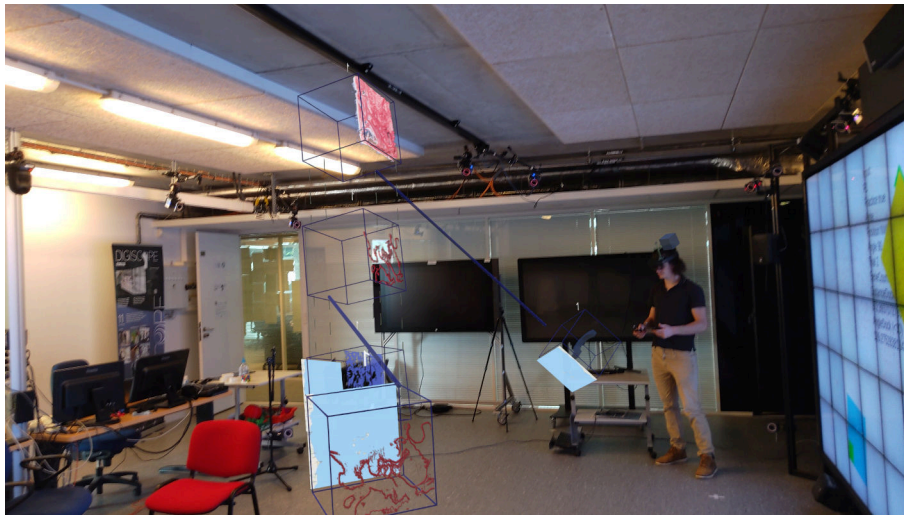
Figure 6.4: Screenshot from one HoloLens of the implementation of the visualization context with the stacked+linked design (Figure 6.1d). All the stacked instances are visible to all the collaborators, but the details of the private linked instances are only visible by their owners. It is to note that this configuration is reaching the limits of the current hardware (i. e., displaying simultaneously four visual instances).
