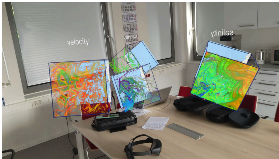
Figure 3.9: A Screenshot taken from the HoloLens showing all the opened properties of the datasets (velocity, salinity, temperature) and their respective instances for the informal evaluation. All the visualizations rely on a Rainbow color scale and use Triangular Gaussian Transfer Functions which weight opacity with (1) the area of interest in the dataset domain (using a Gaussian: Center c and Size \sigma ) and (2) the gradient of the field. From left to right: Velocity magnitude, Temperature (in front), salinity (in back), and salinity again. The labels are orientated similarly in the 3D space for all the users.
