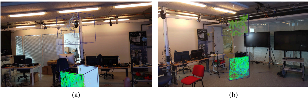
Figure 6.3: Implementation of the subjective views as defined by Figure 6.1b viewed through the AR-HMDs. The highest instance is viewed differently by user A (Figure 6.3a) and by user B (Figure 6.3b). In the implementation, the system creates n personal instances which have the same position, orientation, and scaling. A given user sees only the visual representation he or she owns to not have multiple visible visual representations overlapping each other. I display here the temperature field of the “Cabo Verde” dataset HZG provided me. In the screenshots, some eddies are visually extracted.
