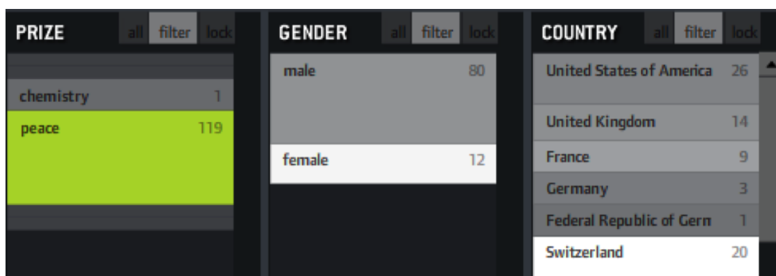
Figure 3.2: Screenshot from three Elastic Lists, each representing a facet. Facet values are represented as rectangles differing in height and brightness to depict the number of objects remaining under each facet value.
